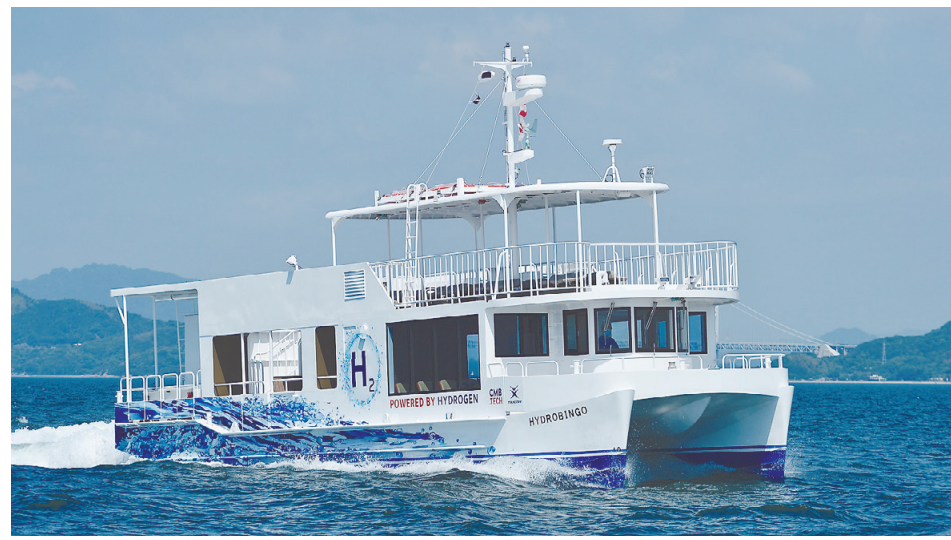
The HydroBingo is the world's first commercial ferry powered by both hydrogen and by diesel engines. This "eco-ship" reduces emissions of carbon dioxide and other harmful gases by up to 50% compared with conventional vessels. TSUNEISHI FACILITIES & CRAFT CO., LTD.
